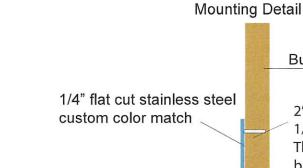
Flush mount to building DO NOT recommend spacers given building facade material and weight of letters. **Building Facade**
