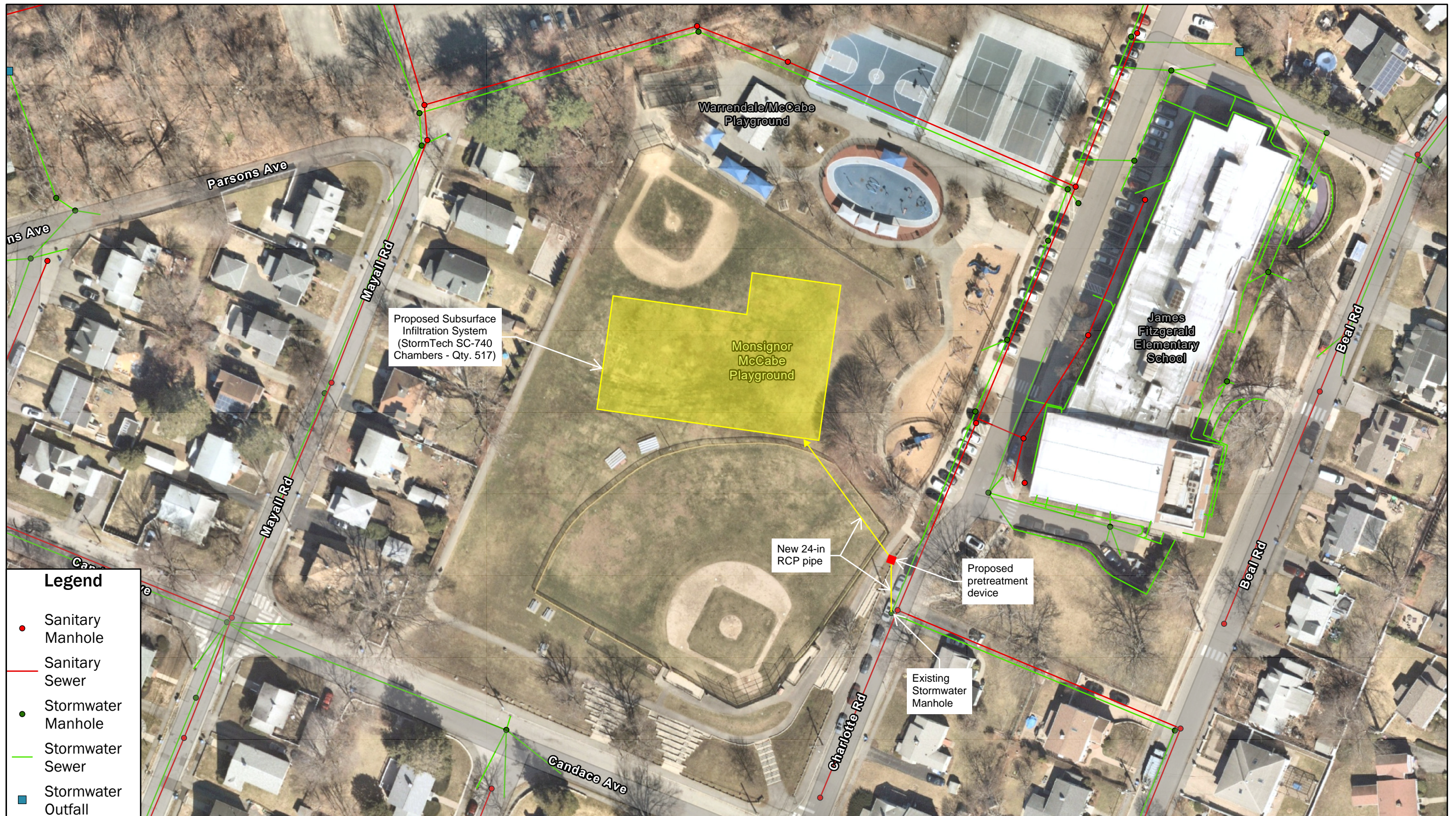
Figure 3. Proposed BMP Conceptual Design Drawing Monsignor McCabe Playground Prepared for City of Waltham by Brown and Caldwell June 2023
