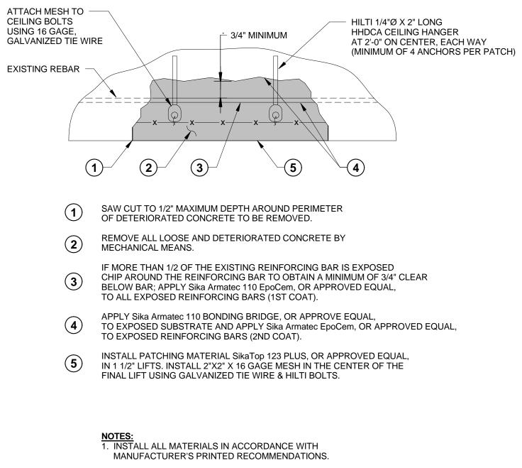
2. IF MORE THAN 25% OF EXISTING REINFORCEMENT IS DETERIORATED, CONTACT ENGINEER BEFORE CONTINUING.
