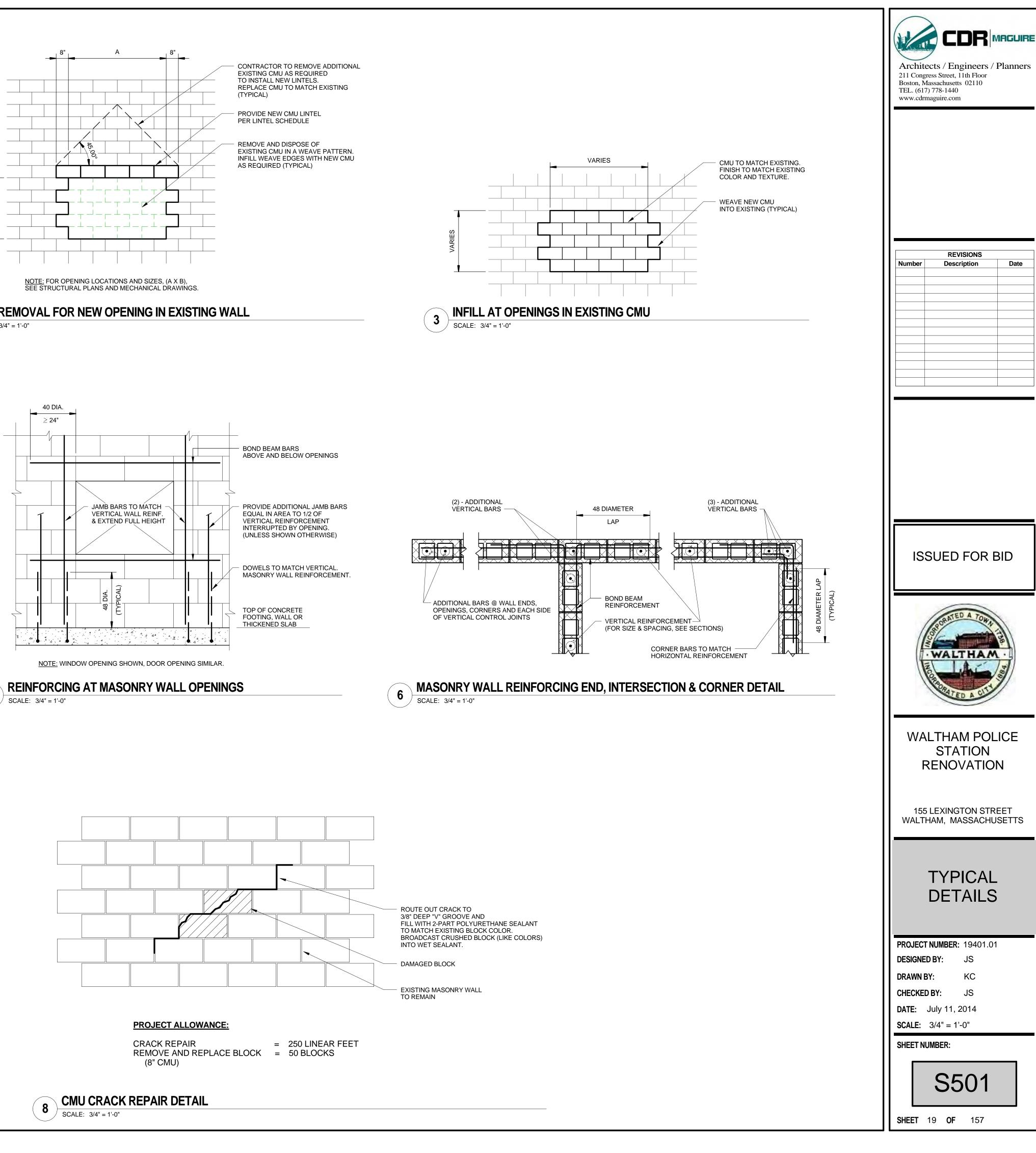
**REINFORCING AT MASONRY WALL OPENINGS** 5
