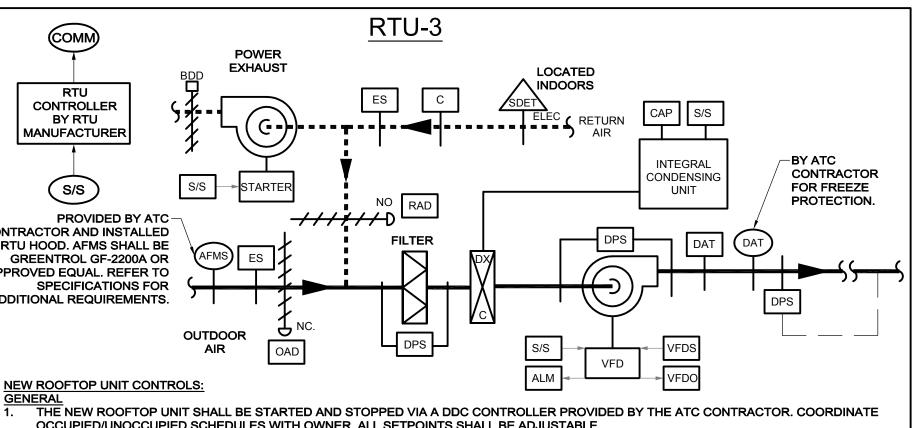
OCCUPIED/UNOCCUPIED SCHEDULES WITH OWNER. ALL SETPOINTS SHALL BE ADJUSTABLE. THE ROOFTOP UNIT ACTUATORS, ENTHALPY SENSORS, DIRTY FILTER SENSOR, DISCHARGE AIR SENSOR, DIFFERENTIAL PRESSURE TRANSDUCER, VARIABLE FREQUENCY DRIVE, AND FROSTAT SHALL BE PROVIDED BY ROOFTOP UNIT MANUFACTURER. THE ROOFTOP UNIT'S REFRIGERATION CYCLE, ECONOMIZER CONTROL, AND SUPPLY FAN VFD OPERATION SHALL BE CONTROLLED BY THE ROOFTOP
