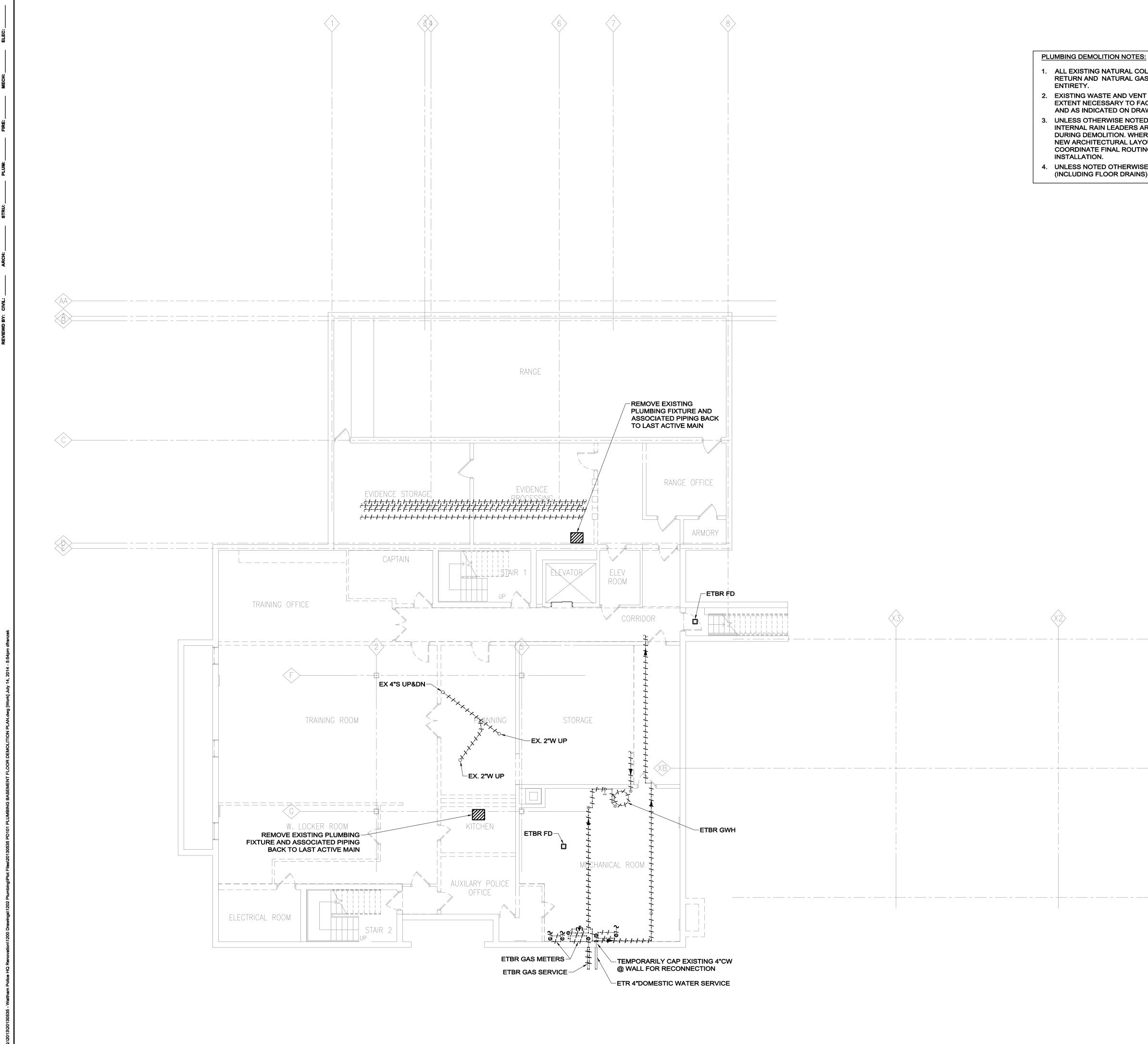
1. ALL EXISTING NATURAL COLD WATER, HOT WATER, HOT WATER RETURN AND NATURAL GAS PIPING SHALL BE REMOVED IN THEIR
