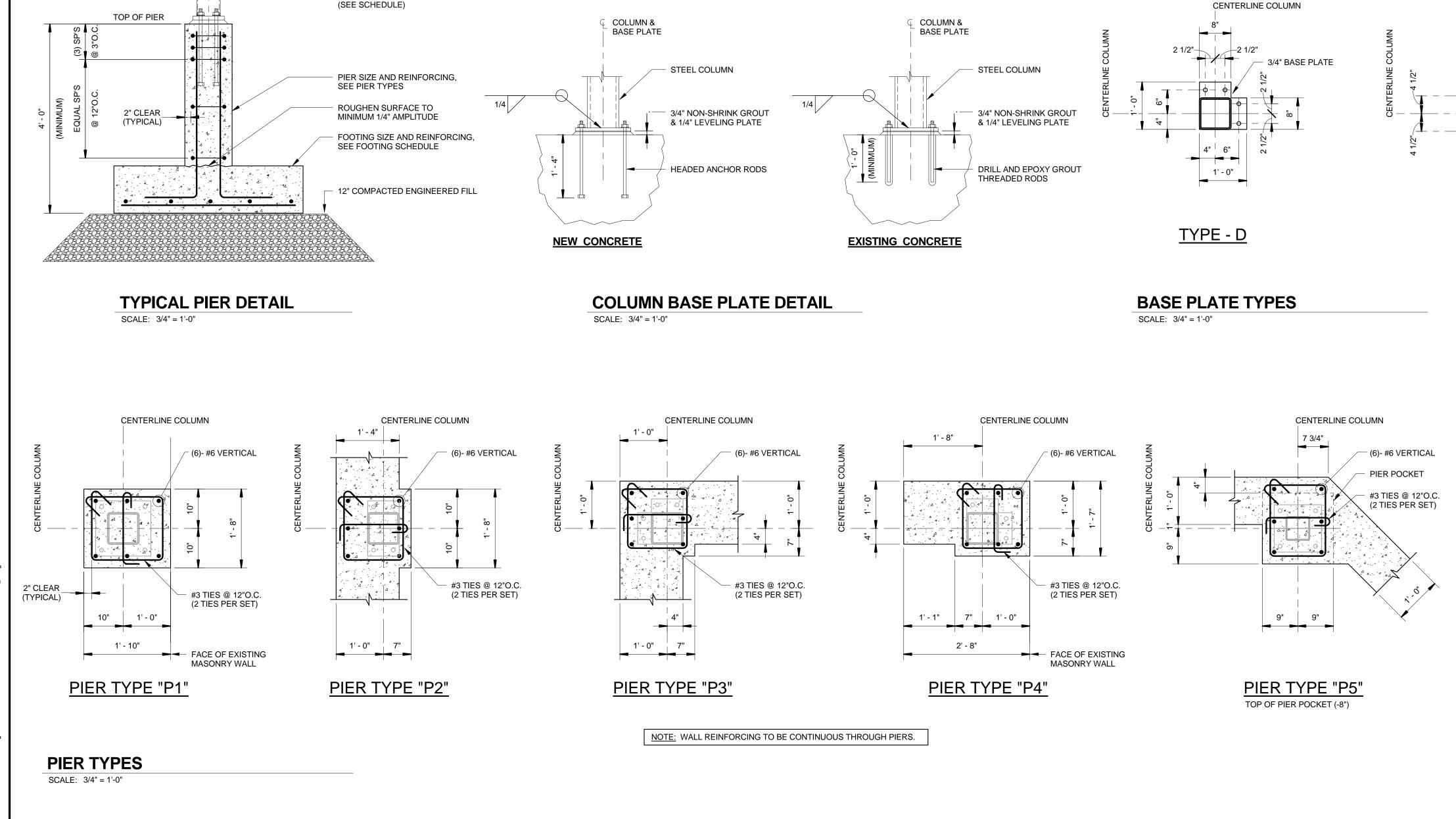
1. ALL COLUMN MATERIAL ASTM A500 GRADE B. 2. ALL BASE PLATE MATERIAL ASTM A572 GRADE 50.
