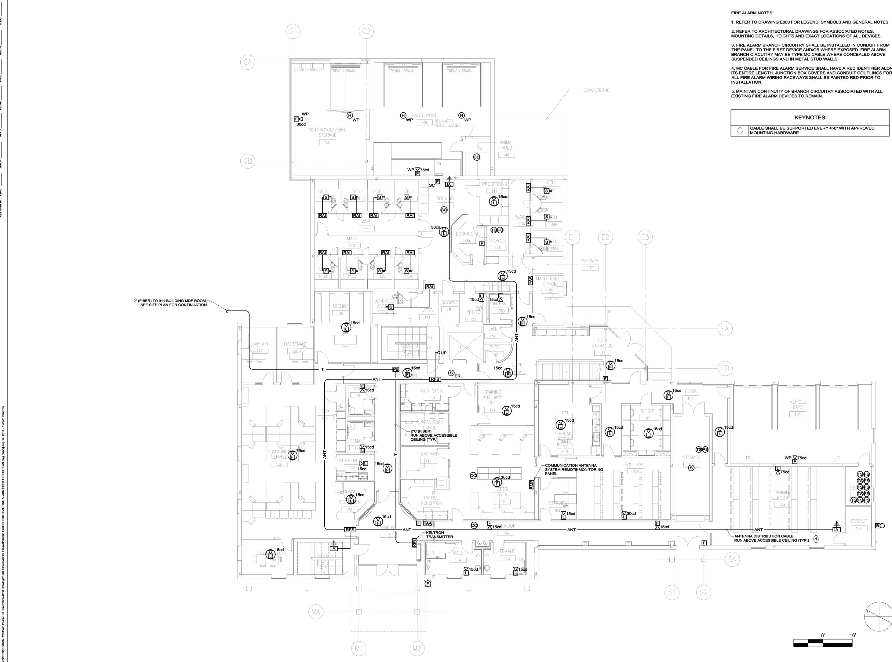
4. MC CABLE FOR FIRE ALARM SERVICE SHALL HAVE A RED IDENTIFIER ALONG ITS ENTIRE LENGTH. JUNCTION BOX COVERS AND CONDUIT COUPLINGS FOR
