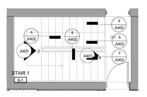
3 ENLARGED STAIR 1 SECOND FLOOR PLAN - EL 12'-8" SCALE: 1/4" = 1'-0"
