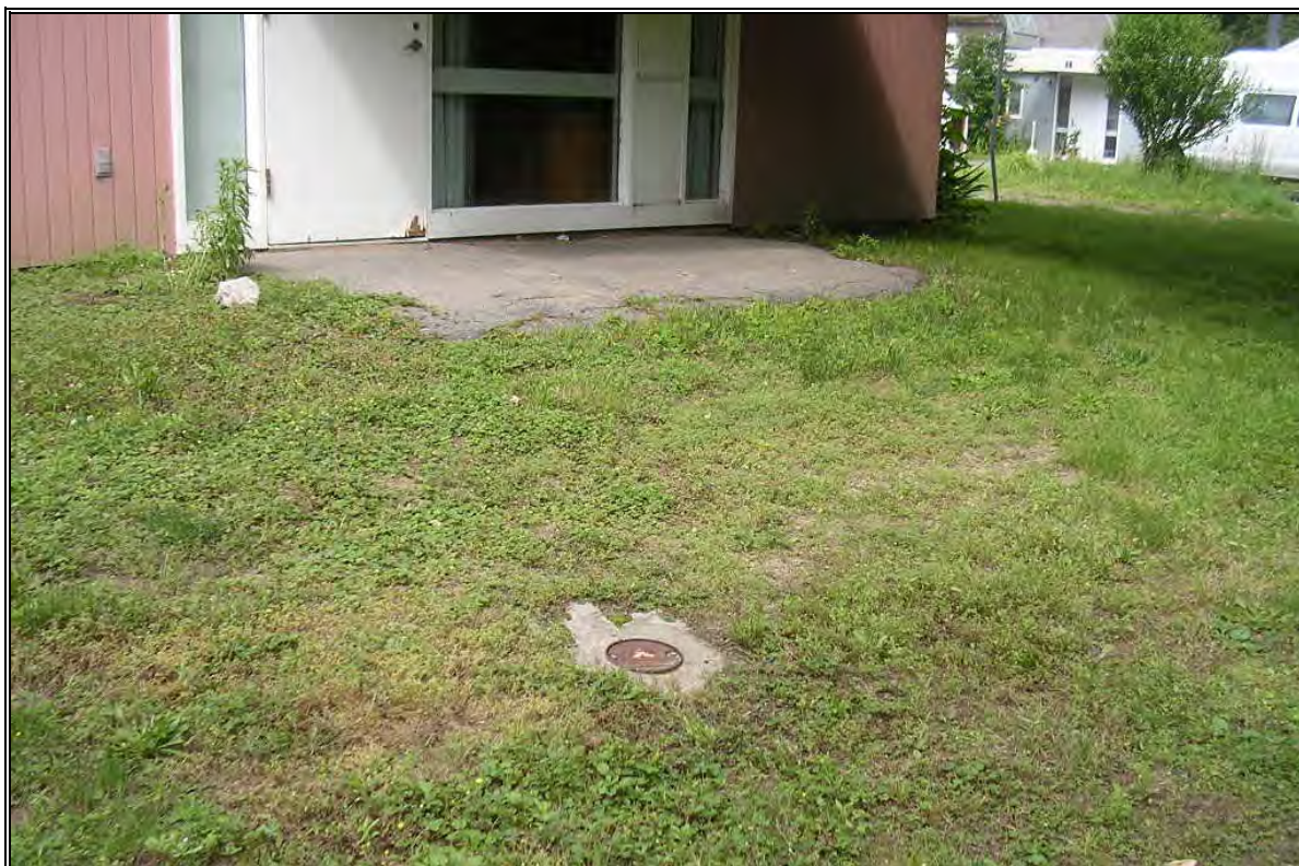
Photo Number 19: Monitoring well CMW-1R outside ICF 23, and location of removed heating oil tank.
