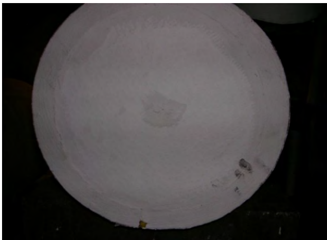
HA 02 White Mud on Fiberglass Caps
