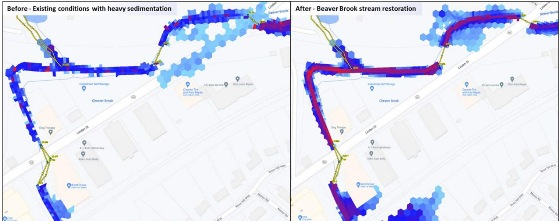
Figure visualizes the 2D model results for the 2-year 24-hour rain event pre- and post-maintenance dredge.
